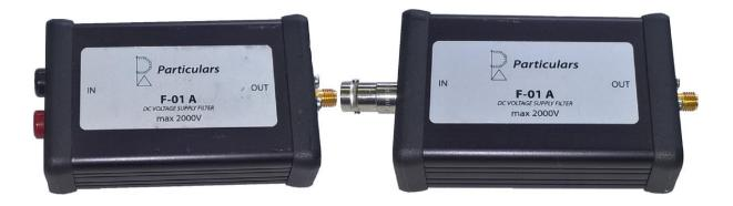
HV filter is an essential part of each system that relies on very stable DC for biasing the detectors. It effectively filters out any high frequency distortions of the DC power supply which would affect the measured signal. It is recommended to use it in any configuration and also for impedance decoupling of individual channels in multi-electrode measurements.
