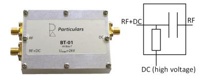
Particulars Bias-T is a decoupling circuitry which enables the connection of high voltage to the readout side. It can stand DC voltages of up to 2 kV (depending on the model).
